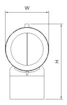
Stainless Steel Ecoflow Venturi Damper c/w Angle Flange
